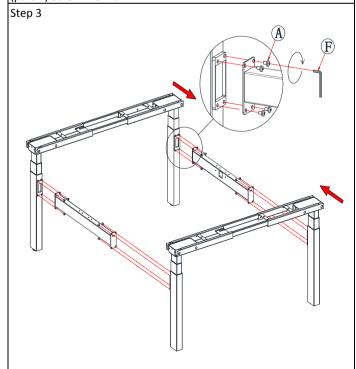
Attach the Side crossbeam (part 7) to the Lifting leg (parts 1 and 2) using (part A) Screw M6x10.
