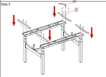
Attach the Side bracket (part 3) to the Crossbeam (part 4) using (part C) Screw M6x45.
