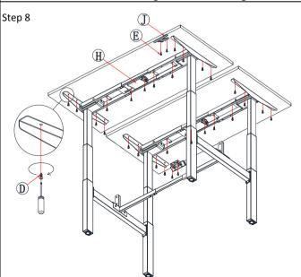
Adjust Crossbeams to the proper position to fit the desktop. Tighten the (part D) Wood screw ST4.8x16 to lock. Attach the Handset (part J) to the underside of the desktop using (part E) Wood screw ST4.2x16.
