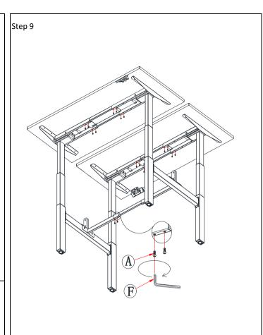
Tighten Crossbeams (part 4) using (part A) Screw M6x10 and tighten Crossbeams (part 5) to the Connecting beam (part 6) using (part A) Screw M6x10.
