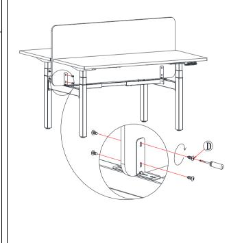
Attach the divider to the L-bracket (part 8). Tighten the L-shape divider bracket using (part D) Wood screw ST4.8x16.
