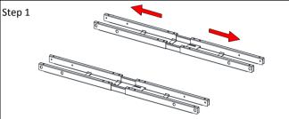
Fully separate the Crossbeams (part 4) you will find the Connecting beams inside.
