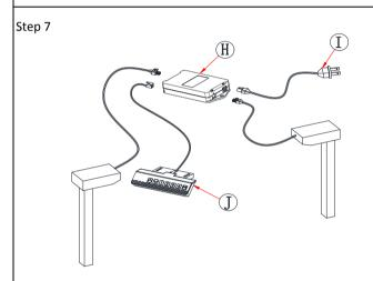
Connect the Lifting legs (parts 1 and 2), Handset (part J), and the Power cable (part I) to the Control box (part H) and plug. Press and hold the UP button until the desk goes to the max height.
