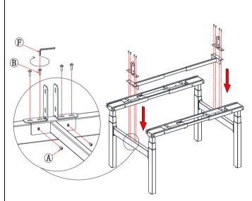
Attach Crossbeam (part 5) to the Side crossbeam (part 7) using (part A) Screw M6x10 and attach L-bracket (part 8) to the Crossbeam (part 5) using (part B) Screw M6x16.
