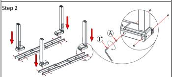
Attach the Lifting leg (parts 1 and 2) to the Crossbeam (part 4) using (part A) Screw M6x10.
